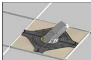
3. Insert the down light through the cutted hole.
